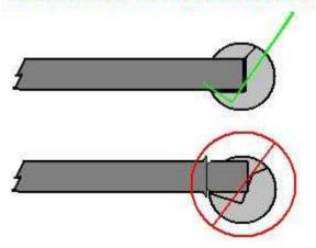
Wrong adjustment can wear the lifter rod making it flared and difficult to remove from case
